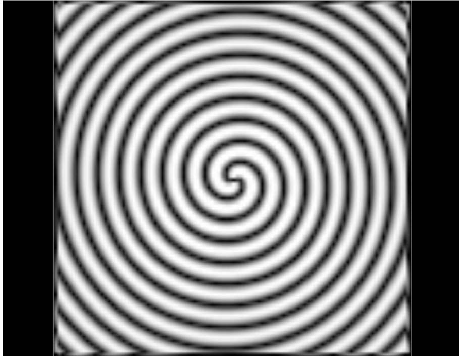
Fig 3. The Electric Potential showing the double spiral of charge layers.
